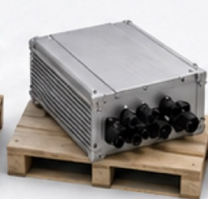
3 ELECTRONICS BOX 850 x 520 x 250 mm ~35 kg
