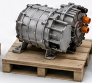
2 REAR E-DRIVE UNIT 850 x 650 x 550 mm ~110 kg
